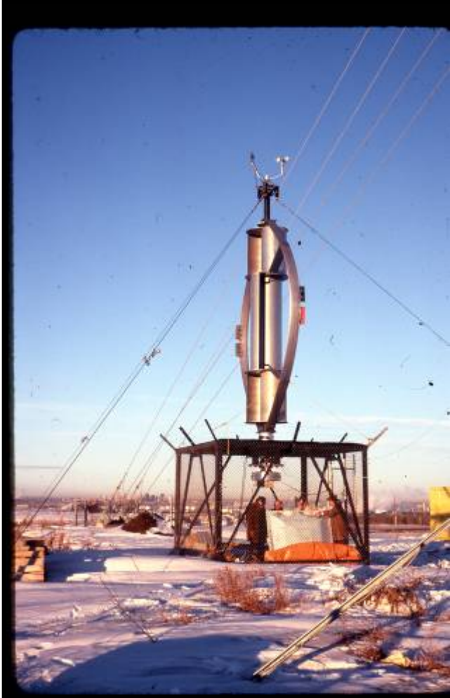
Figure 4 - Testing a vertical axis wind turbine manufactured by Bristol Aerospace LTD. near Edmonton, Alberta.
