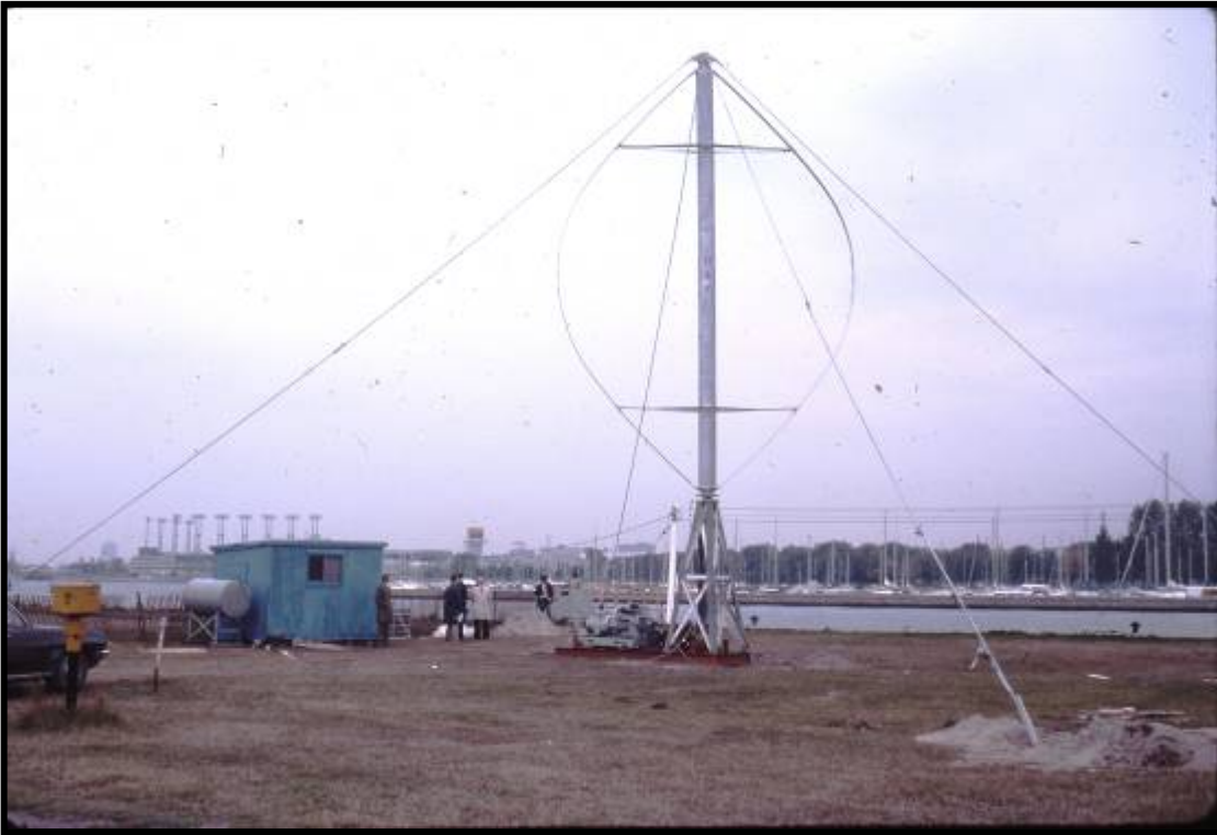
Figure 7 - Testing a vertical axis wind/diesel hybrid on Toronto island in September 1977.
